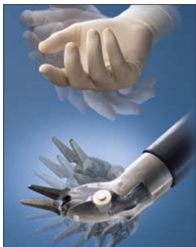
The da Vinci robot has EndoWrist® instruments that can rotate 360 degrees. This allows for a wider range of motion, more intricate suturing, and greater precision and dexterity than human fingers.
