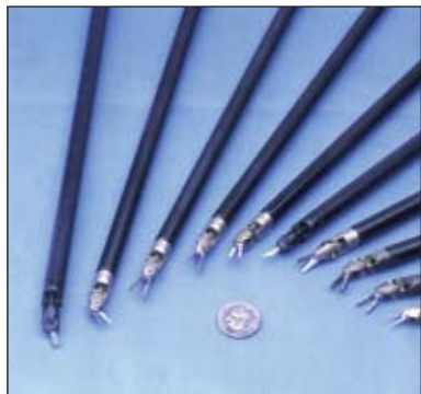
EndoWrist® instruments offer intuitive motion, finger tip control, and tremor reduction.
